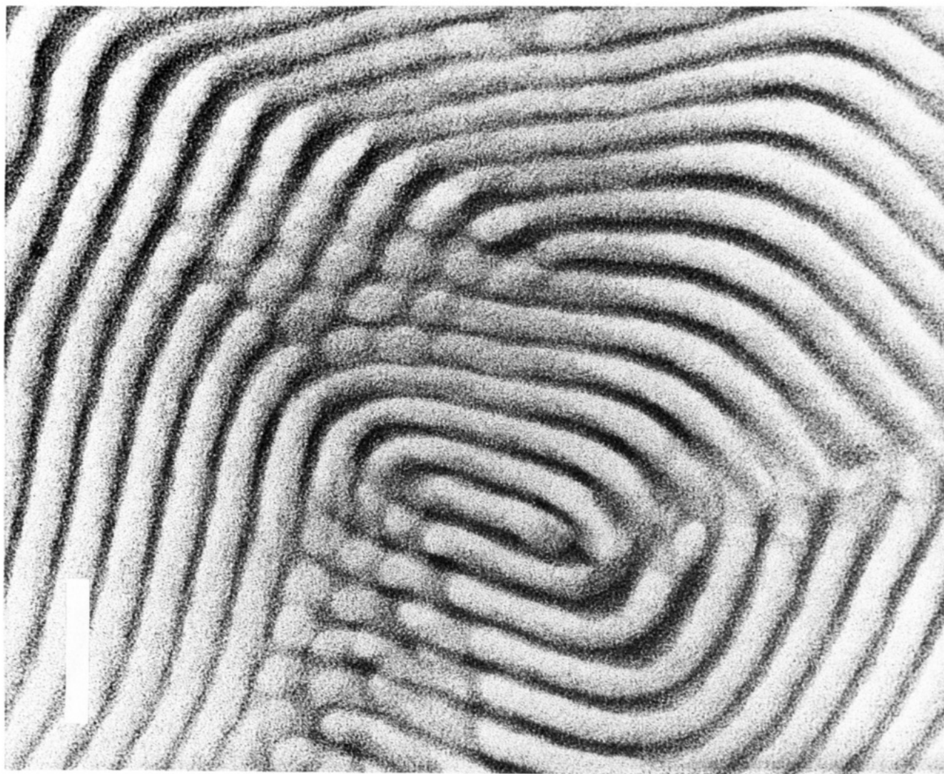
Figure 7. Bright-field TEM of [(\text{ZnPh})_2(\text{bTAN})]_{80}/[\text{MTD}]_{250} ; bar = 1000 Å.
